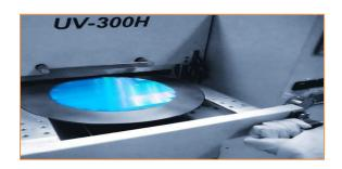
Fig. 2UV-Ozone cleaner for 200 mm or 300 mm wafers [12]
